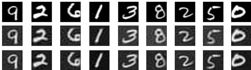
Figure: Top row: Nine samples from the MNIST [5] test dataset, shifted horizontally randomly by up to six pixels. Middle row: Output of a linear equivariant autoencoder designed to be equivariant under horizontal translations. The network architecture is determined by the integer vector \mathbf{r} . Bottom row: Output of a dense linear autoencoder with r = 99 without equivariance imposed.
